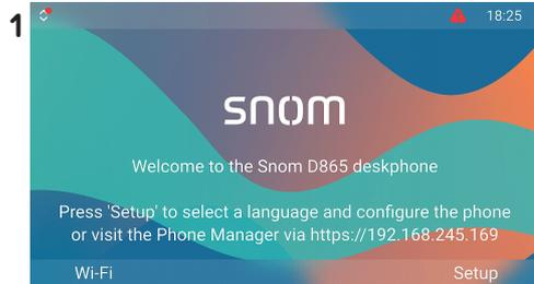
When the phone has been connected, it will show the welcome screen with the IP address of the **Phone Manager**. It is more convenient and therefore recommended to perform the first time setup using the **Phone Manager**. Enter the *IP address* into the browser's address bar on a computer in the same network as the phone.
