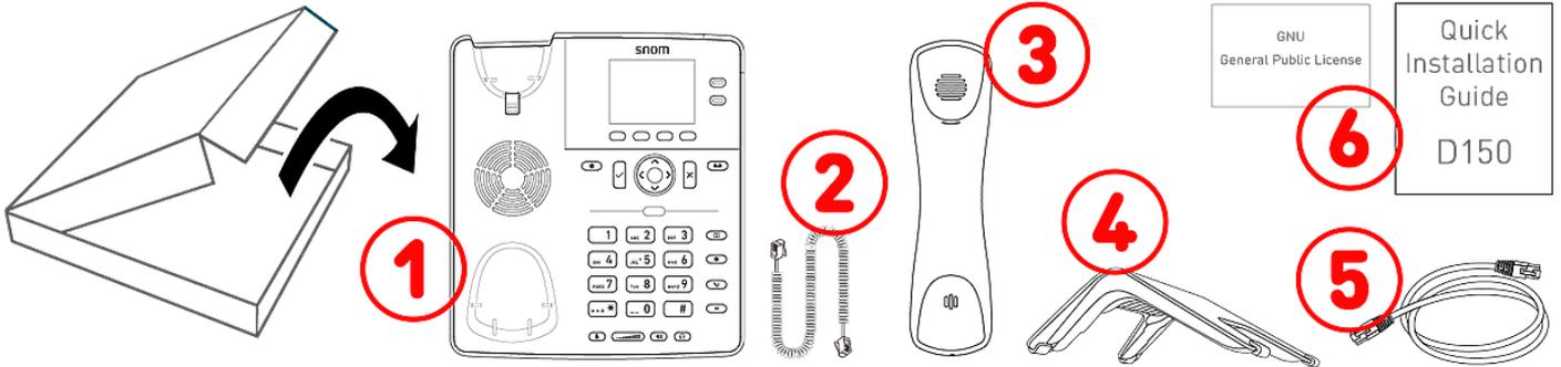
**A-1:** IP desk phone D150 | **A-2:** Handset cord | **A-3:** Handset | **A-4:** Footstand | **A-5:** Ethernet cable: 1.5 m | **A-6:** Documentation
